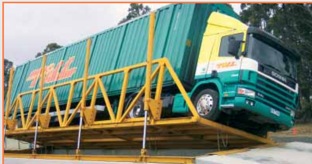
Picture: Tilt test conducted at the Australian Automotive Research Centre in Anglesea Victoria. Please note that no vehicles inside the Maxibox were damaged during the tilt trials.
